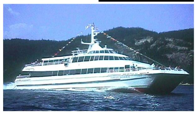
When launched in 1995, the engines in the Canadian fast ferry "Famille Dufour II" were rated at a modest 1640kW each which enabled the twin HamiltonJet HM811 propulsion system to produce thrust for a speed of 30 knots with the vessel lightly laden (refer |etBrief No.266 August 1995). However, upgrading work on the engines during the northern winter of 1996 boosted the power output to 2088kW a piece, which has resulted in fully laden speeds in excess of 35 knots.
