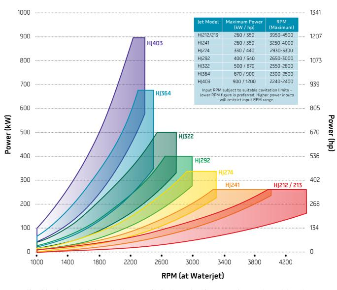
Note: Waterjet selection is determined by a range of hull and operational factors, most importantly vessel size and displacement (weight), and not necessarily by matching the above specifications to the desired engine power/RPM curve. In all cases you should consult HamiltonJet for assistance with waterjet selection.
