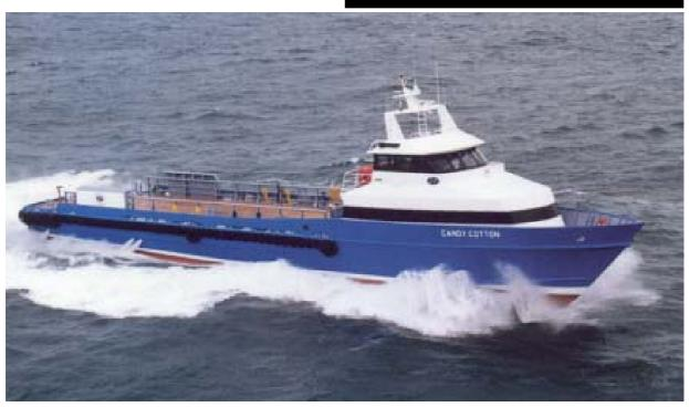
With oil exploration moving further offshore, crew boat charterers require larger vessels with greater speed and cargo carrying capacity. Service company Candy Fleet operates a series of 44-metre crew boats, each of which utilises a single Hamilton Jet HM571 waterjet propulsion system to supplement a quadruple setup of conventional propellers.
