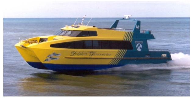
New Zealand eco-tourism company Dolphin Discoveries (1996) Ltd. have launched a new jet powered catamaran vessel. Based in the Bay of Islands, "Discovery IV" is a 17.7 metre Teknicraft design, powered by twin Hamilton Jet Model 362 jets directly driven by Caterpillar 3406E diesel engines.
