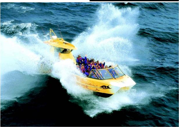
"SuperJet" is an apt description for this 10 metre Hamilton Jet powered excursion craft operating on Lake Taupo in the centre of New Zealand's North Island. Twin model 241 jets provide thrust for a maximum lightship speed of 42 knots, dropping only slightly to 39 knots when fully fuelled and loaded with 31 passengers.
