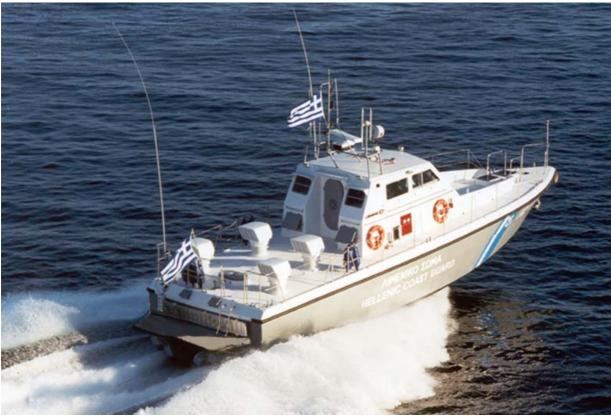
A fleet of 16 new high speed patrol craft for the Greek Coast Guard will all be powered by Hamilton waterjet propulsion systems. Each of the 17.4 metre craft will have twin Model HM422 jets directly driven by MTUV12 diesel engines.
