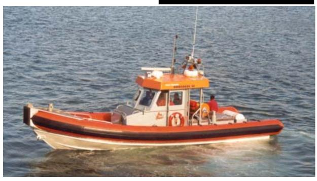
Belgium operator Ship Support Technics has purchased a Hamilton Jet powered RIB craft for salvage and rescue work around the Belgian coastline. The "Ribworker 38", built in the UK by Ocean Dynamics, is powered by a single Model 321 waterjet driven by a Scania DSI 9 diesel engine through a ZF gearbox and has a top speed of 33 knots.
