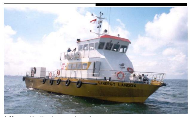
A 28 metre Hamilton Jet powered crew boat for servicing oil rigs in Asia has been delivered to its owners, Sanergy Marine of Singapore. Twin Hamilton model HM571 waterjets driven by Caterpillar diesel engines through ZF gearboxes push the vessel, which has a displacement of 71 tonnes, to a top speed of 25 knots. The jets were supplied as an integrated package including intake and transition duct, hydraulic power supply and
