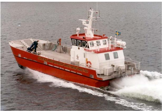
The Södertörns Fire Fighting Brigade of Sweden has recently taken delivery of a new Hamilton Jet powered Jetcat 19 catamaran for fire and rescue duties. Built from aluminium by Swedish builder Capo Marin AB, the vessel incorporates twin Hamilton Jet Model HJ391 jets powered by Scania diesels.
