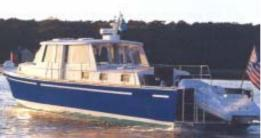
• Waterjet propulsion – Twin Hamilton HJ321 waterjets provide outstanding efficiency, reliability, acceleration, and manoeuvrability, as well as low noise and vibration.
