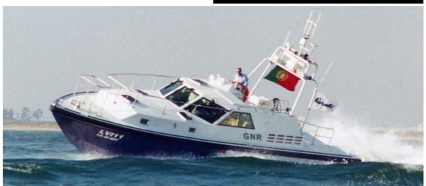
When the marine branch of the Portuguese Customs Service up-graded its patrol fleet with a 12 new 16-metre vessels, twin Hamilton Model HJ391 Waterjets were chosen as the best propulsion option. Designed to combat the increase in smuggling from North Africa, the new boats have been designed with many seakeeping and safety features.
