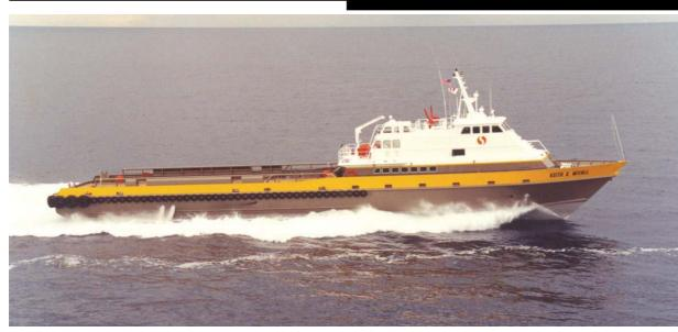
Oil rig crew/supply boats operating in the Gulf of Mexico today need to be fast, reliable and manoeuvrable, both when empty and when carrying a full load of passengers and cargo. SEACOR Marine's latest vessel, Keith G. McCall, fits all these criteria with performance to spare, due largely to its propulsion package of quadruple Hamilton Model HM811 waterjets.
