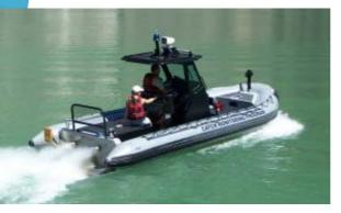
preferred. However, in this application the owners required a vessel that could transfer to ocean use if required. The jet features hydraulic controls for both steering and reverse functions.
