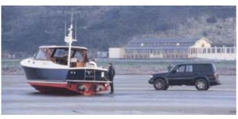
The waterjets are also an advantage on the extensive tidal flats of The Netherlands. With its shallow draft and no risk of damage to the propulsion gear, the Riffler can be safely beached to wait for the next tide to come in.
