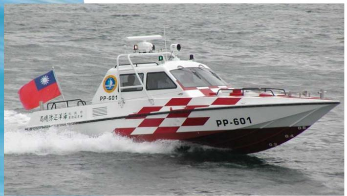
TYPE: PP-601 SERVICE: Fast Patrol Craft LENGTH: 9.50 metres (LOA) **BEAM:** 3.00 metres **DRAUGHT:** 0.55 metres **CONSTRUCTION:** FRP SPEED: 45 knots WATERJETS: Twin HamiltonJet Model HJ274 **ENGINES:** Twin Yanmar diesel engines Model 6LY-STP, each 275kW (370hp) @ 3300rpm **GEARBOX:** ZF 220 **OWNER/OPERATOR:** Taiwan Coast Guard, Taipei, Taiwan **DESIGNER/BUILDER:** Lung Teh Shipbuilding Co., Taipei, Taiwan HamiltonJet DISTRIBUTOR: Port King International Co Ltd, Taipei, Taiwan
