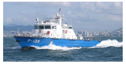
The Korean Coast Guard's flagship vessel was designed for a maximum speed of 45 knots using twin HM811 waterjets and 3600hp MTU engines.
